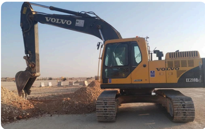
Volvo EC210B excavator during excavation works
